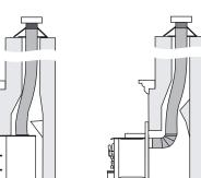
3a) Full Flue Liner (No Cleanout Required)
